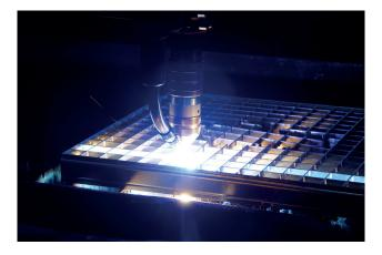
The FineFocus 800 can be modified quickly and easily for applying the HotWire technology. Electrically conductive, nonconductive, combined and interrupted materials e.g. gratings, armoured concrete or wired glass can be cut with this technology.
