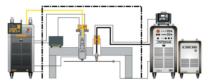
Connecting system: Usable on guiding system such as our PreciTrack/NCT system in combination with plasma cutting unit.
