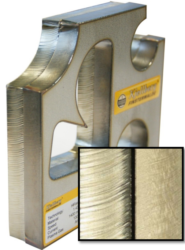
Comparison underwater cut and dry cut 10 mm stainless steel
